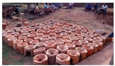
From 2016, RDIS opted for another stove liner-Rural wood stove that is well used in Uganda, the stove passed highly with 29.4% thermal efficiency in respect to Improved Cook Stoves for East Africa (ICSEA) water boiling test and safety test. This picture shows the stove under the process of installation; its body is made of mud bricks, after the burning boxes are fixed
